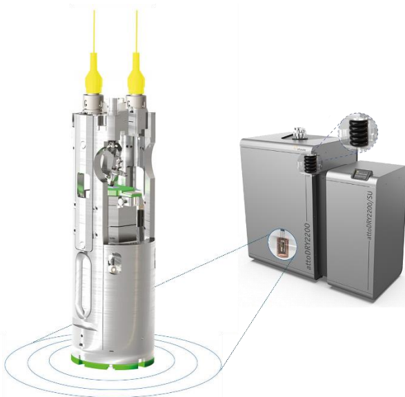
Fig 2: Experimental setup for cryogenic MFM imaging. The attoAFM I microscope, operated in MFM mode, is mounted inside the attoDRY2200 closed-cycle cryostat, which provides a vibration-damped environment with base temperatures down to 1.7 K and vector magnetic field control.
