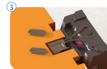
Perform the cantilever exchange; alignment grooves on chip guarantee perfect positioning.
