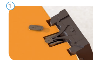
Put the cantilever holder into the exchange basis.
